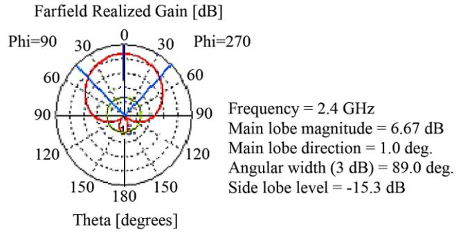
Fig. 7 Radiation pattern at f = 2.4GHz (Enhanced)
