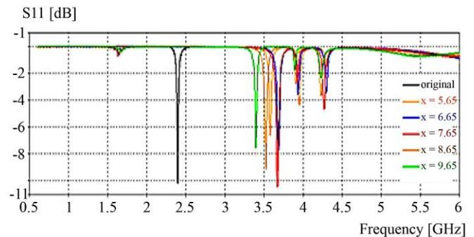
Fig. 14 Reflection Loss for different ring slots dimensions
