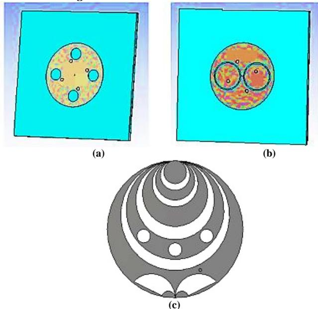
Fig. 13 Patch antenna with (a) circular slots, (b) Cylindrical ring slots, and (c) fractal slots
