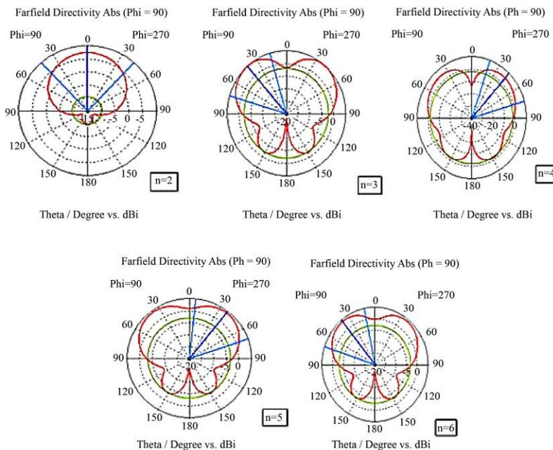
Fig. 10 Radiation pattern for various numbers of Vias "n"
