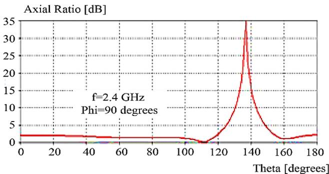
Fig. 6 Axial ratio at f = 2.4GHz (Enhanced)
