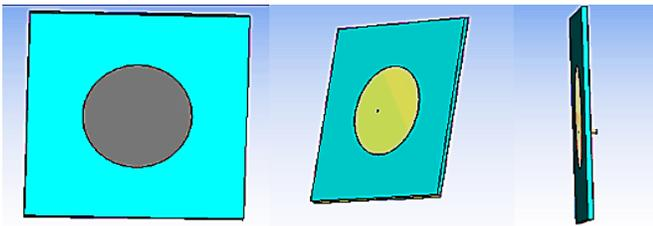
**Fig. 1 Circular patch operating at 2.4 GHz**
