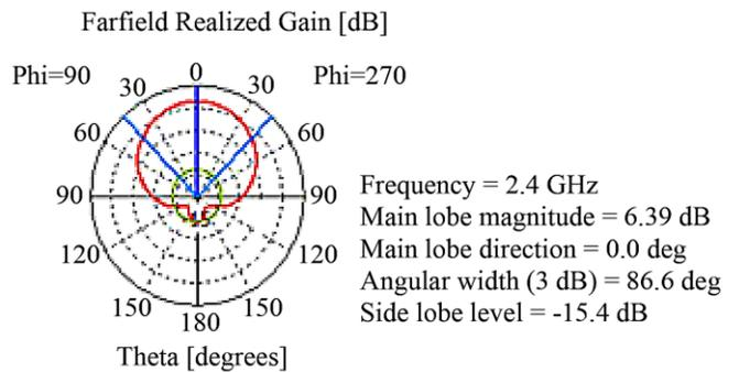
**Fig. 4 Radiation pattern at f = 2.4GHz (Reference)**
