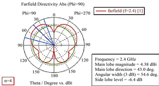
Fig. 12 Radiation Pattern for the optimum design
