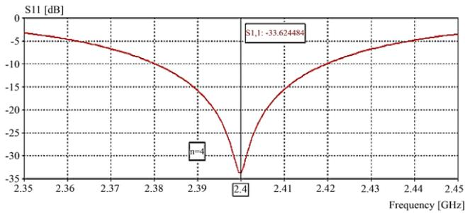
Fig. 11 Reflection loss for the optimum design
