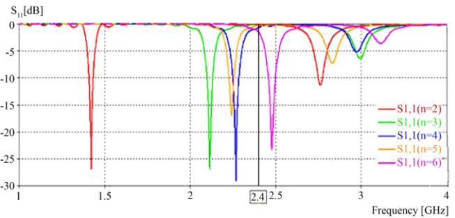
Fig. 9 Reflection loss vs frequency for various numbers of Vias "n"
