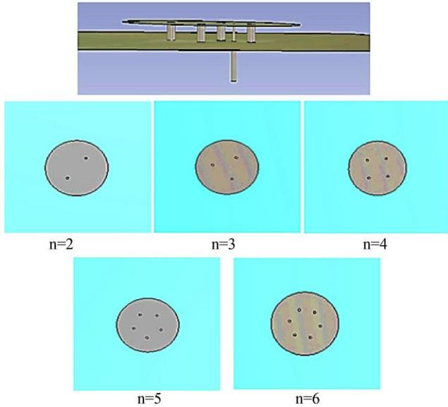
Fig. 8 Patch antenna with vias (Top and Side View)
