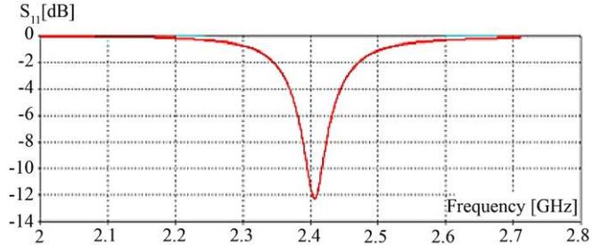
**Fig. 2 Reflection loss vs frequency (Reference)**
