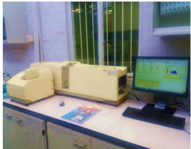
Fig. 2 Malvern 2000G PSD analyzer
