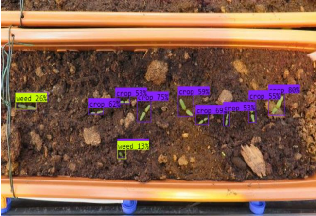
Fig. 6 (b) Real-time weed and crop object detection with IoU visualization – Sample 2. Figure (a) and (b) show images with bounding boxes for weed and crop classes. This visualization is crucial for informed weed removal and crop yield estimation.
