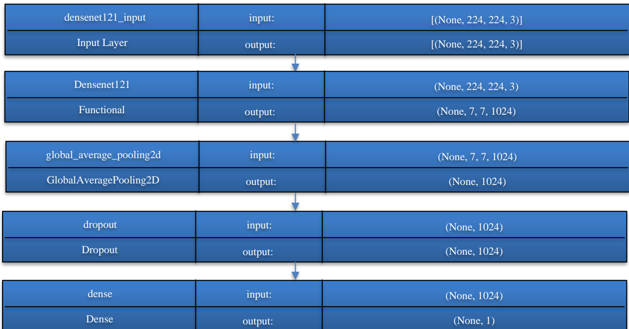
Fig. 3 An overview of the proposed model architecture based DenseNet121
