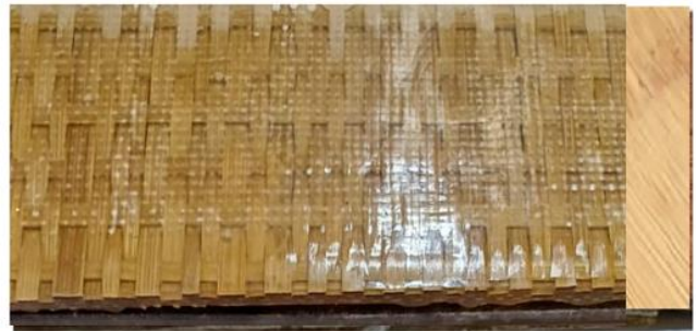
Fig. 2 Laminate composites reinforced hybrid fiber musa acuminata stem fiber (MASF)-bamboo fiber (BF) with a polyurethane resin (PR) matrix
