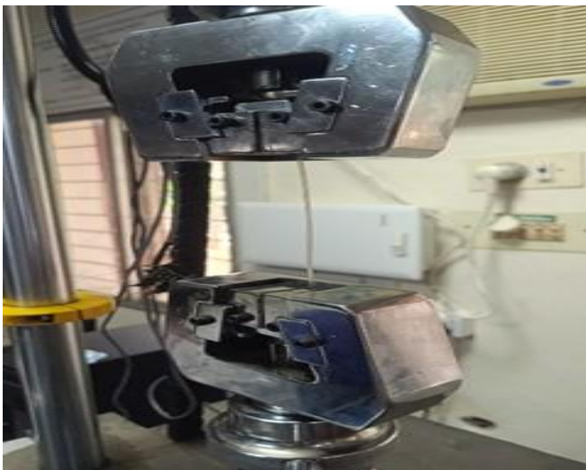
Fig. 3 Tensile testing of composite filament
