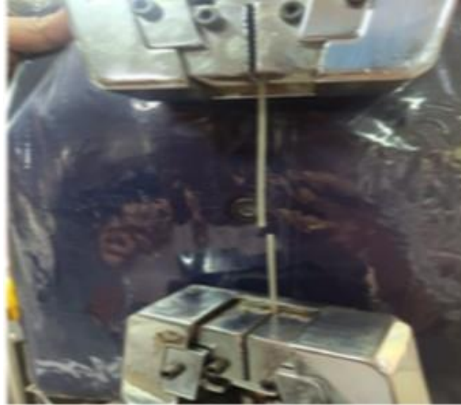
Fig. 12 a) Filament failure under tensile loading
