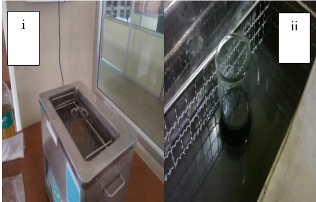
Fig. 1 (a) Bath type Sonicator for formulation of conglomerates: i) nTiO 2 with base oil ii) nMoS 2 with base oil
