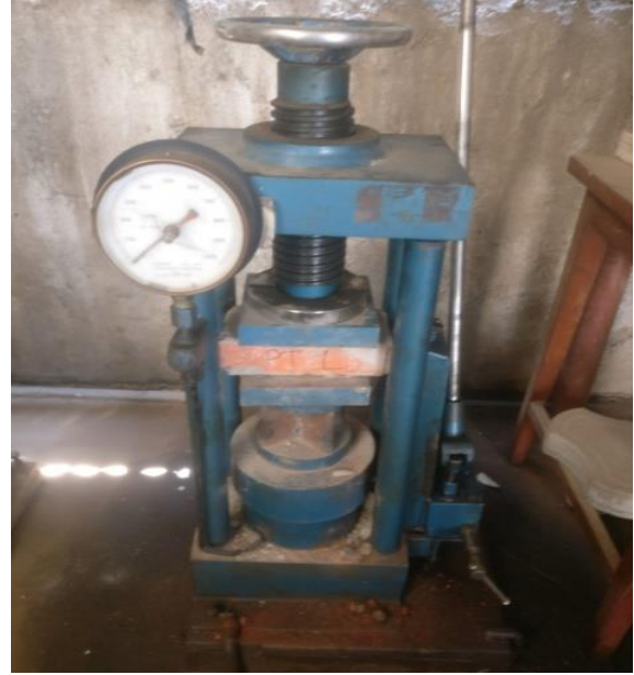
Fig. 11 Brick compression test
