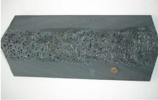
Fig. 1 Polycarbonate and polyethylene plastic with fibreglass composite sleeper [3]
