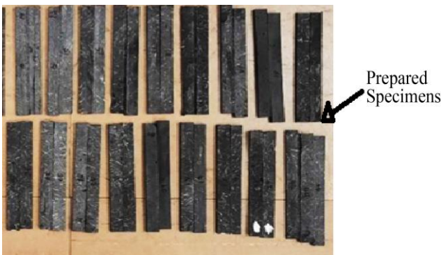
Fig. 5 Samples used for vibration and damping test
