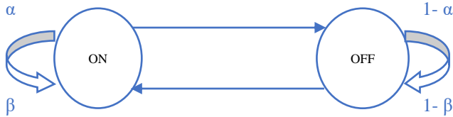
Fig. 7 Model for describing the behavior of next-hope sensor node analogous to channel sensing state as ON/OFF
