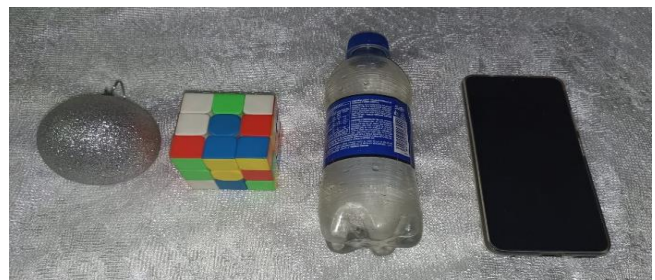
Fig. 6 Objects used for the grip tests, in the shape of sphere, cube, cylinder and flat rectangular (from left to right)
