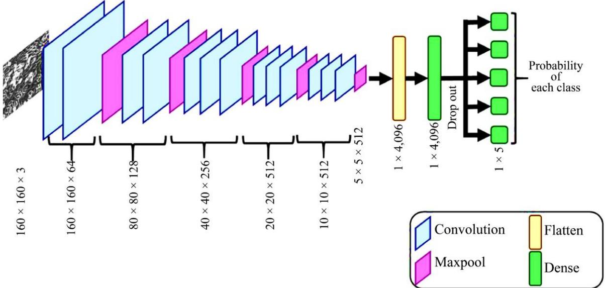
Fig. 5 Architecture of pre-trained TF models (a) VGG16 (b) VGG19 (c) Resnet50
