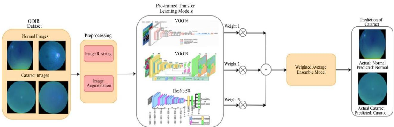
Fig. 1 Algorithm of proposed ensemble model
