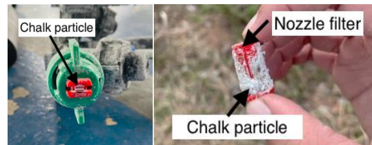
Fig. 6 Clogged nozzle from fertiliser spraying
