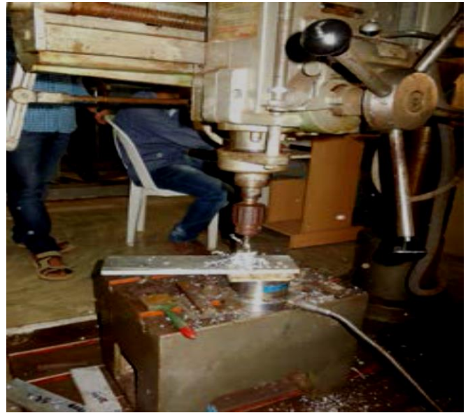
Fig. 5 (a) Experimental setup with KISTLER dynamometer
