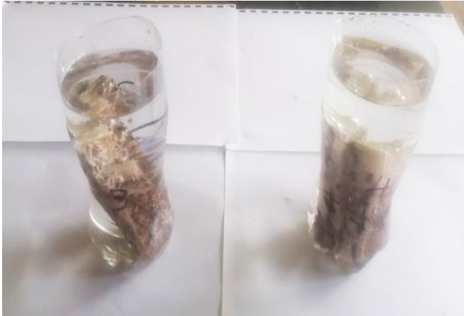
Fig. 4 Samples completely submerged in NaOH solution for chemical resistance test
