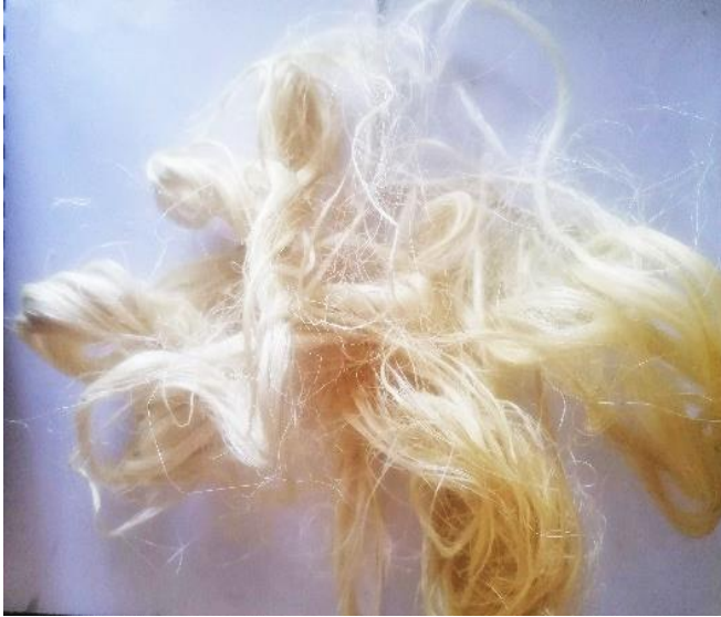
Fig. 3 Mercerized sisal fibres
