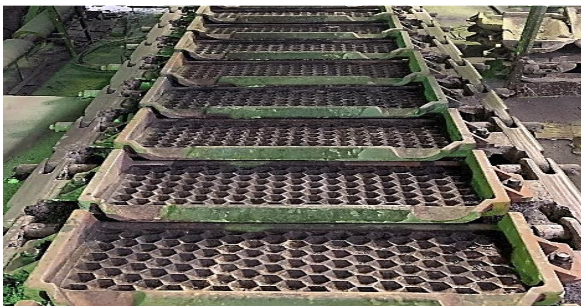
Fig. 4 Casting machine equipped with cellular casting moulds
