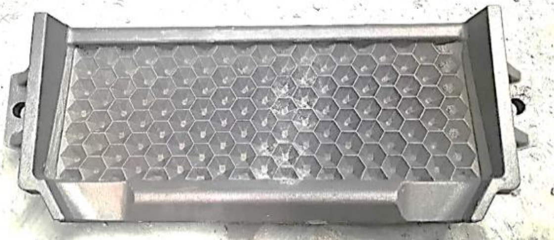
Fig. 2 Experimental cellular casting mould
