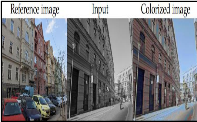
Fig. 5 Image coloring by example technique
