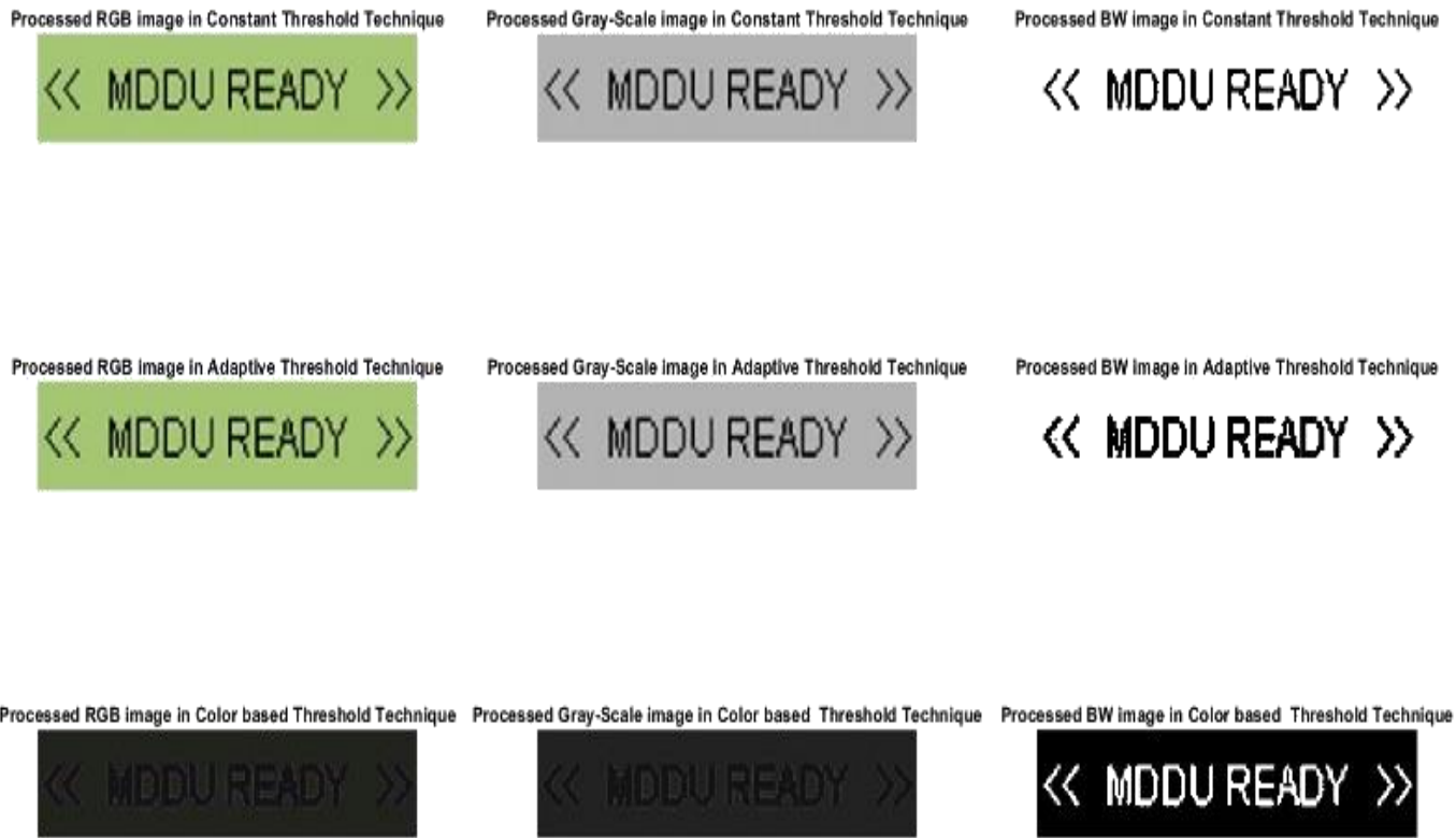
Fig. 7 Resulted in a Text message for “<< MDDU READY>>”, obtained through all three RGB to BW conversion methods
