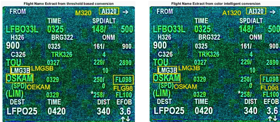
Fig. 18 output of Text messages (Yellow) from the Bulk Text # 1 Sub Panel, obtained through the threshold and Color Intelligent RGB to BW conversion methods
