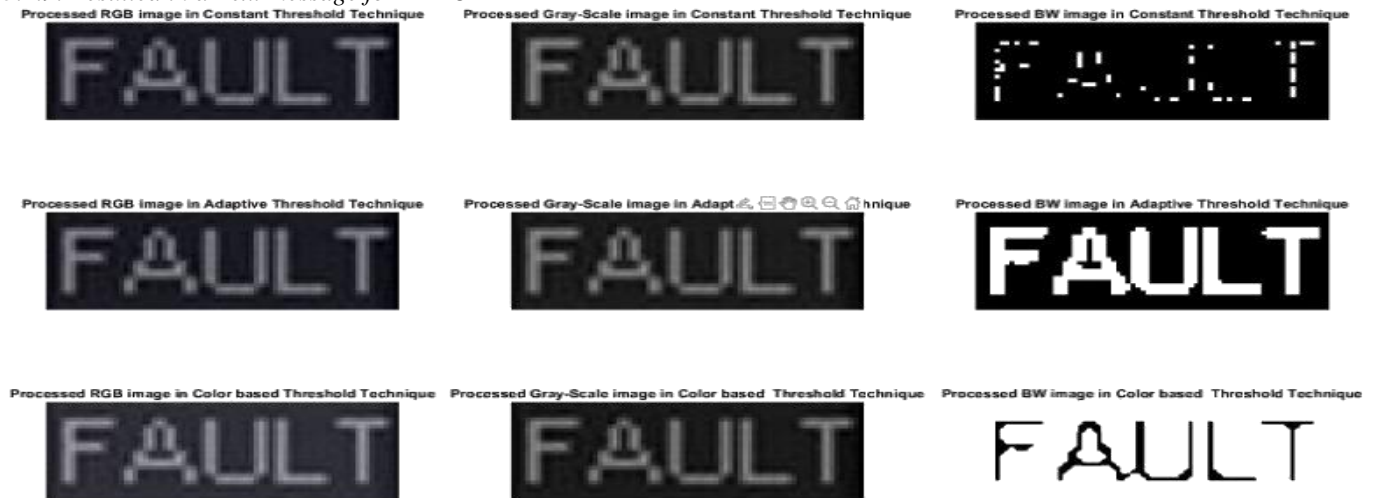
Fig. 12 Resulted in a Text message for "FAULT", obtained through all the three RGB to BW conversion methods
