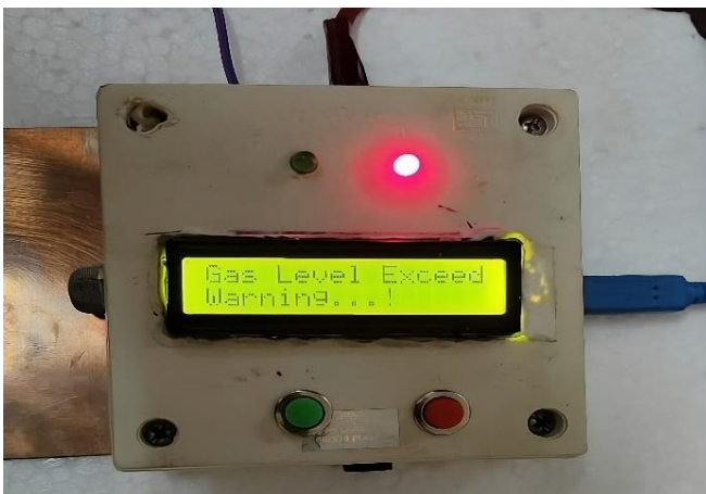
Fig. 7 Gas Leakage detects
