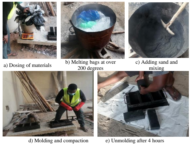
Fig. 4 Pavers making process
