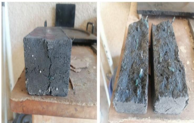
Fig. 11 Appearance of improved pavers after tensile failure
