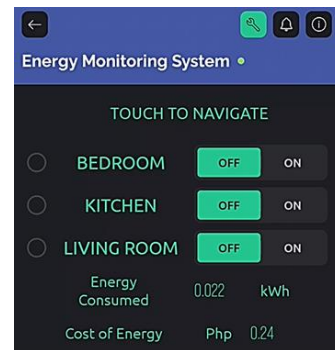
Fig. 7 Displayed values of energy consumption and cost in the mobile application
