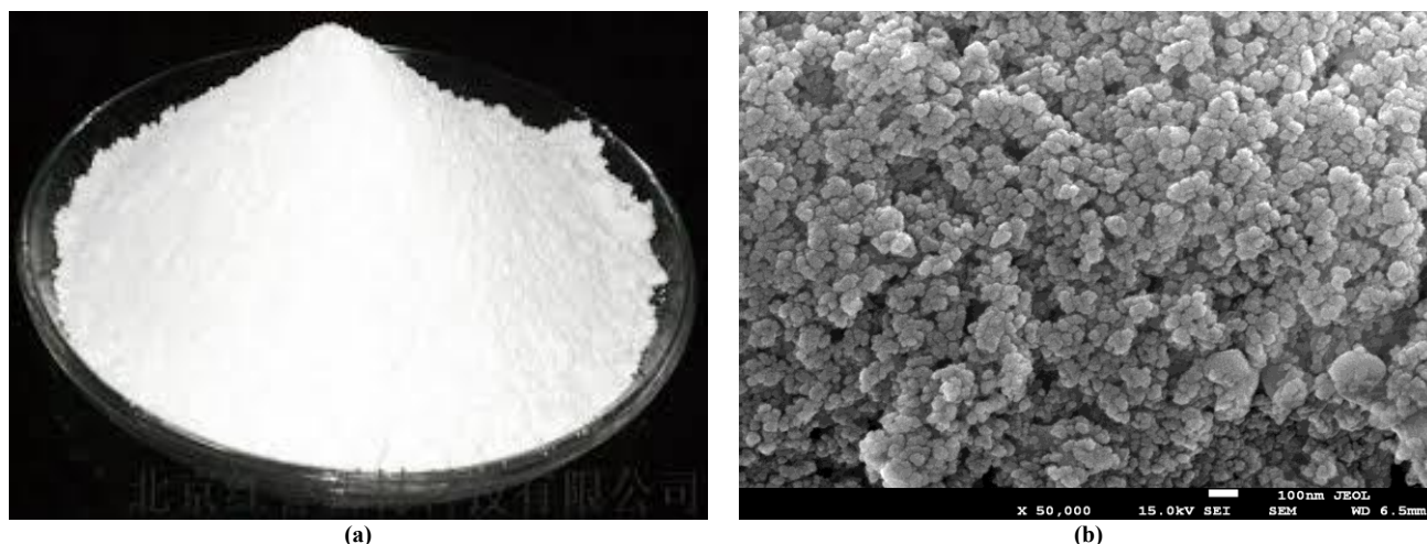
Fig. 3 Al 2 O 3 nanoparticles: (a) As-received powder, and (b) SEM morphology showing nanoscale agglomerates.
