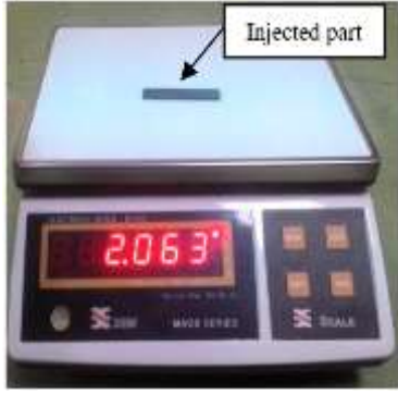
Fig. 3 Weighing of the injected part on a digital scale
