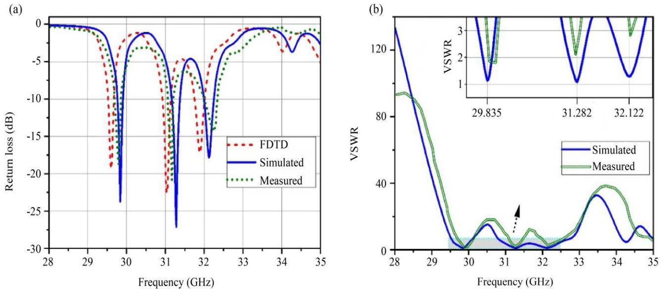
**Fig. 10 (a) Simulated, Measured, and FDTD return loss (S<sub>11</sub>), and (b) Simulated, Measured VSWR measurements**
