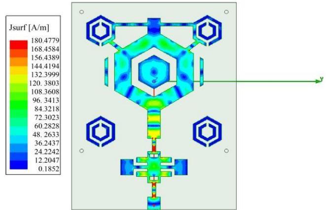
Fig. 6 Surface current density of proposed filtering antenna
