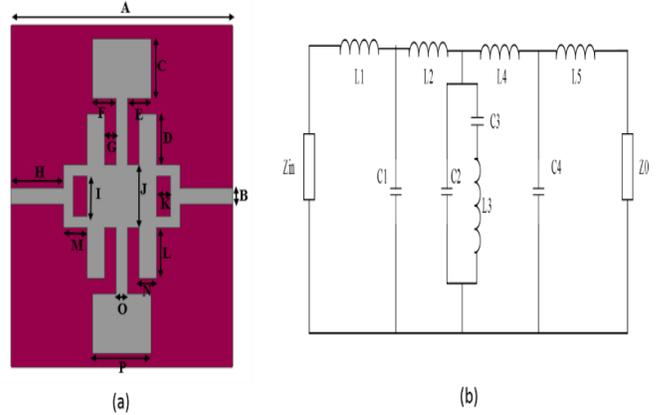
**Fig. 4 (a) Band pass filter design, the values are A=9.5mm, B=0.5mm, C=1.9mm, D=1.65mm, E=1mm, F=1mm, G=0.5mm, H=2.25mm, I=1.3mm, J=2mm, K=0.6mm, L=1.65mm, M=1mm, N=0.75mm, O=0.5mm and P=2.5mm, (b)Equivalent circuit of bandpass filter where L1-L5: inductances and C1-C4: capacitances**
