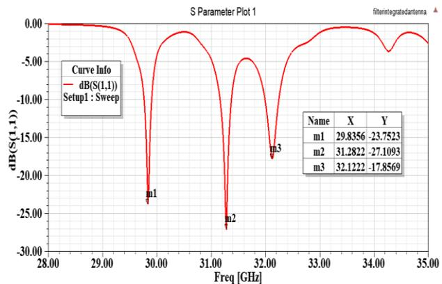
**Fig. 3 Return loss (S11) vs frequency of filtering antenna**
