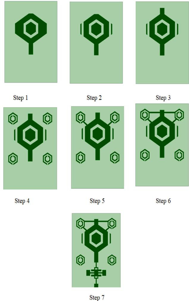
**Fig. 2 Design Evolutions of Simulated Antenna Model**
