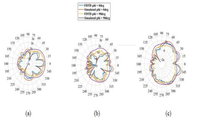
Fig. 7 The radiation pattern for simulated and FDTD at (a) 29.835 GHz, (b) 31.282 GHz, and (c) 32.122 GHz
