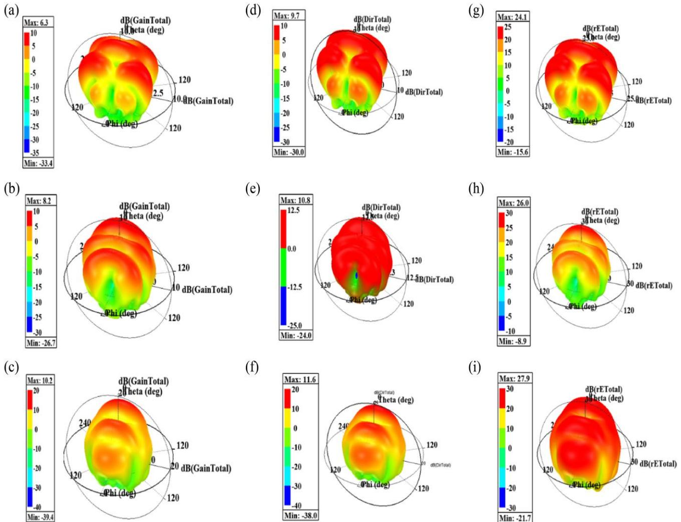
Fig. 8 (a-c) Simulated performance analysis of 3D gain plot, (d-f) 3D directivity plot, (g-i) 3D radiation pattern plot, for (a,d,c) 29.835 GHz, (b,e,h) 31.282 GHz, and (c,f,i) 32.122 GHz, respectively
