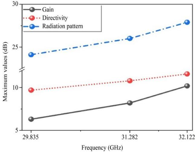
**Fig. 9** The maximum values obtained for gain, directivity and radiation pattern from the data shown in Fig. 8
