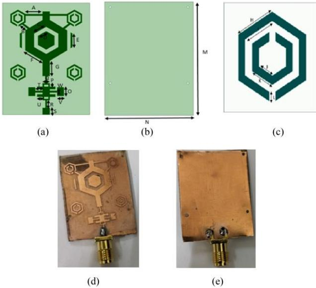
**Fig. 1 Proposed filtering antenna (a) Top view (b) Bottom view (c) HSRR (d) fabricated prototype Top view and (e) Bottom view of fabricated prototype**
