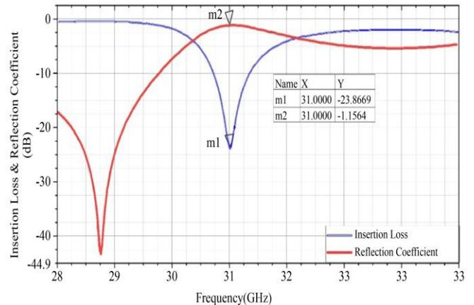
**Fig. 5 Performance analysis of filter design: reflection coefficient and insertion loss**
