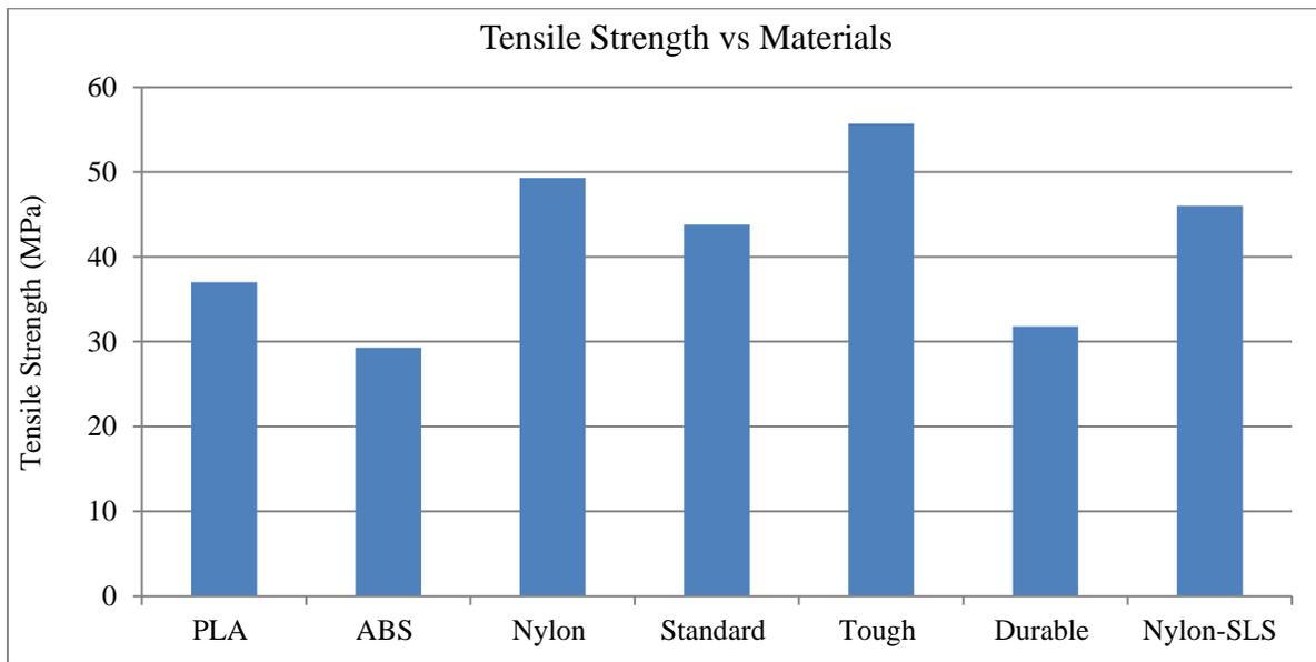
Fig. 14 Materials tensile strength
