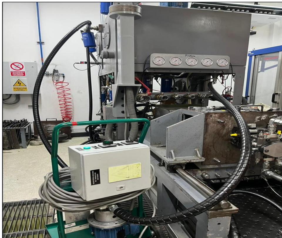
Fig. 11 Oil cleaning on the test stand - Bosch Rexroth
