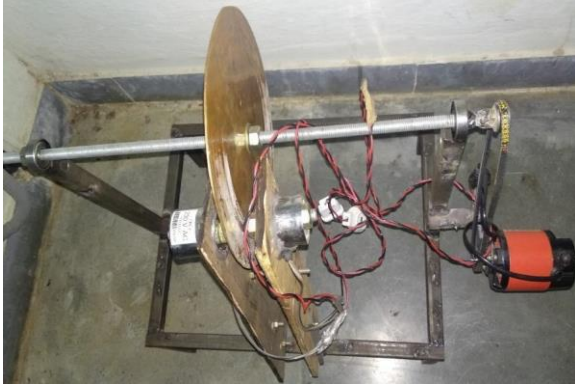
Fig. 5 Electromagnetic braking system with copper
