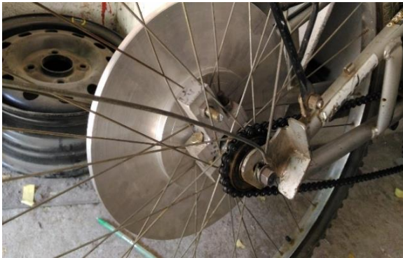
Fig. 6 Electromagnetic braking system with Aluminum
