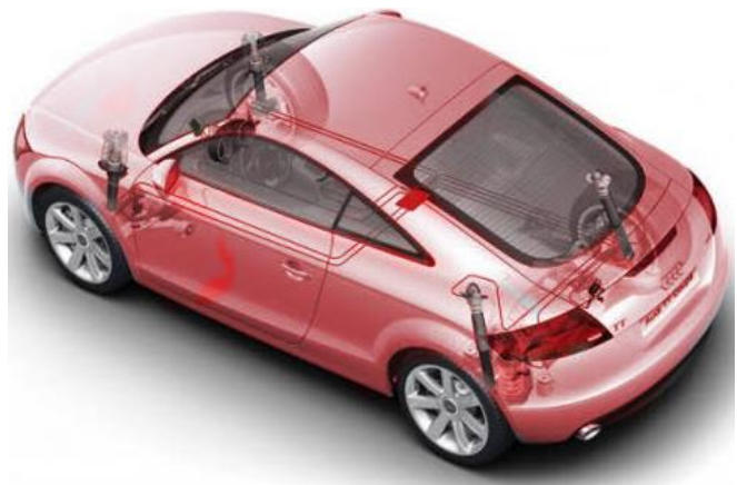
Fig. 9 MR fluid dampers in Audi TT [41]
