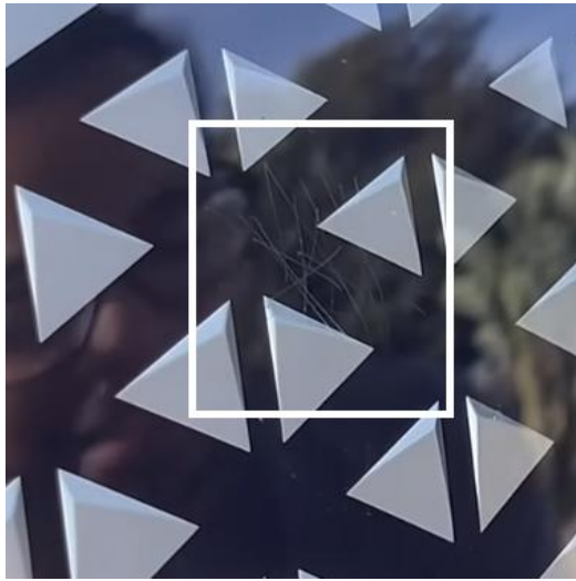
Fig. 10 (b) BMW iX grille with scratches [43]
