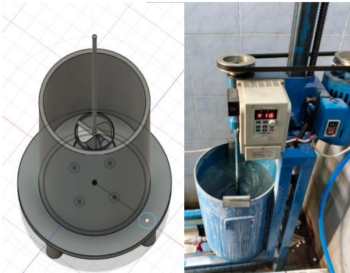
Fig. 6 ASTM C1138 underwater abrasion test apparatus (source: author documentation)
