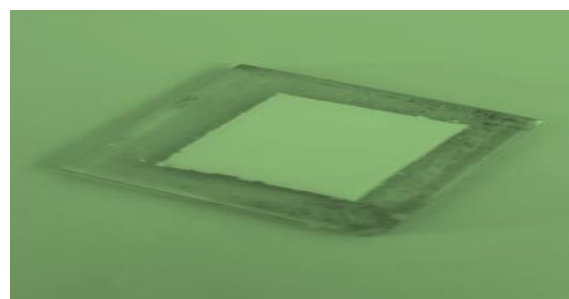
Fig. 1(a) FTO coated glass fixed with paper tape, and (b) Thin film of \text{TiO}_2 on FTO-coated glass after spin coating.
