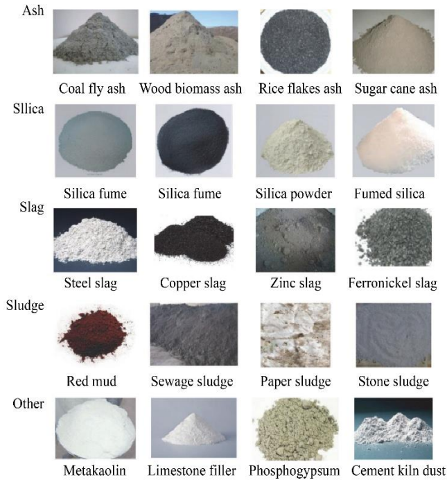
Fig. 5 Supplementary cement replacement materials [7]
