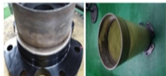
Fig. 2 Failure of high-speed shaft coupling due to insufficient bonding strength
