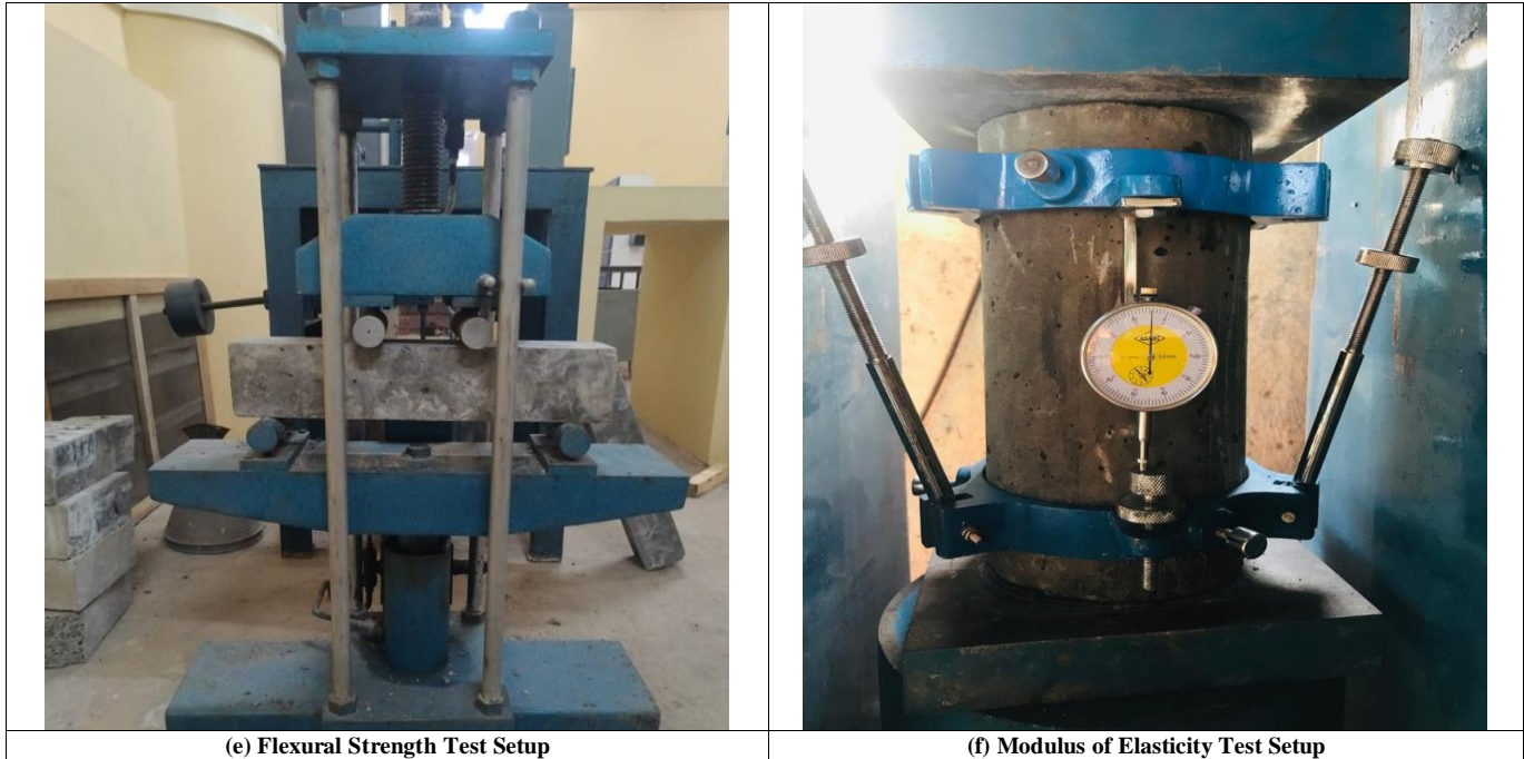
Fig. 10 (a) Compression strength specimen, (b) Split tensile strength specimen, (c) Rapid chloride penetration test, (d) Water penetration test specimen, (e) Flexural strength test setup, and (f) Modulus of elasticity test setup.
