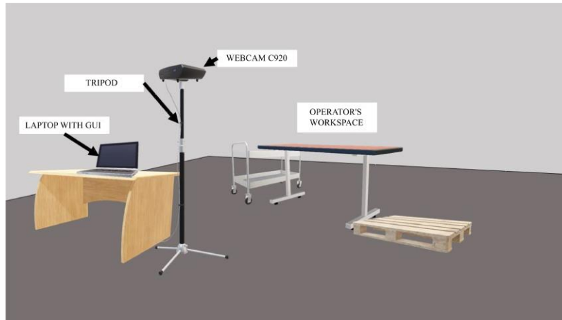
Fig. 3 Experimental Setup; 3D design layout of the project in assembly line
