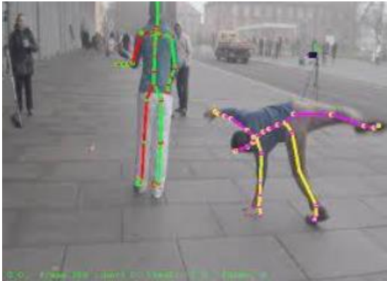
Fig. 2 Marker-Less visual using camera vision [8]
