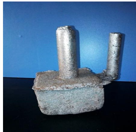
Fig 7: Cast produced using sprue height below the critical drop height
