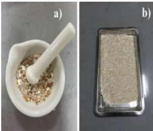
Fig. 2-a Minging apparatus Fig. 2-b Granulated egg shell (GES)
