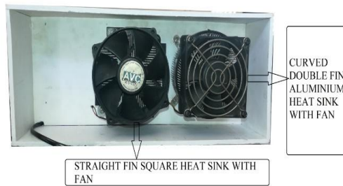
Fig 2.4 Rear View of Thermoelectric Air chiller
