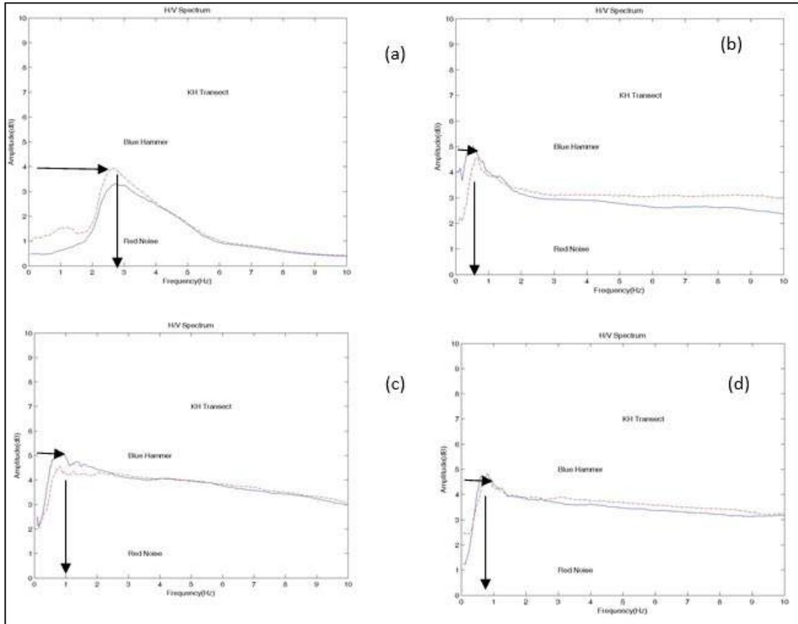
**Figure-3:** Shows H/V spectral ratios in thick alluvial soil cover and deeper bed rock formation along (a) Nagavali fault zone passes near Dusi village, (b) Vamsadara fault zone passes Lukalam village, (c) Konnada-Kumilini fault zone crossing near Kustira village and (d) Brahmoni fault passes through Baitarani River/Jutana village along transect. The figure shows high amplification at low frequency.
