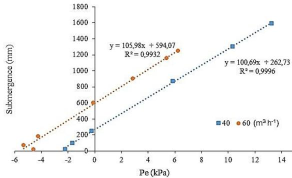
Fig. 4. The 6" pump constant flow rate obtained in the regression equation
