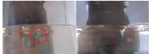
Fig. 6. In the 6 " pump vortex images at 40 (a) and 60(b) m<sup>3</sup> h<sup>-1</sup> flow
