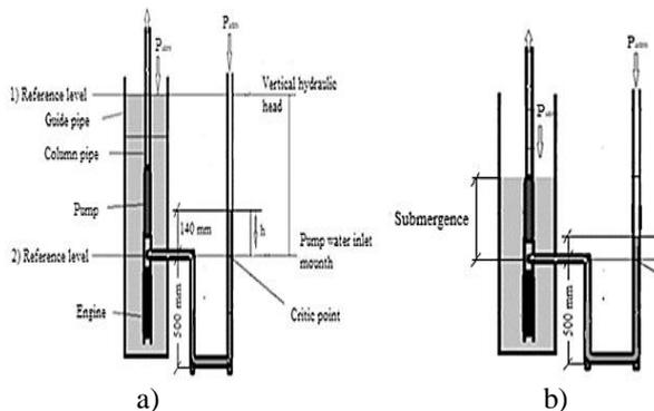
Fig.1. View of U tube differential manometer in different operating situations (a) state at the time the pump is not running b) state at the time the pump is running).
