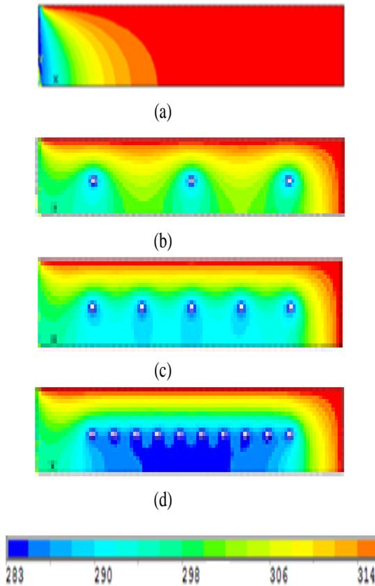
Fig. 8. Temp. distributions inside the wall a) without pipes b) 3 pipes c) 5 pipes and d) 10 pipes
