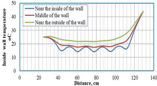
Fig. 11. Variations in temperature of the inside wall for various positions of pipes within the wall
