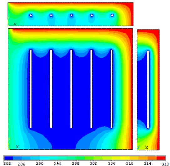
Fig. 6. Temperature distributions within the wall for five pipes at the wall center
