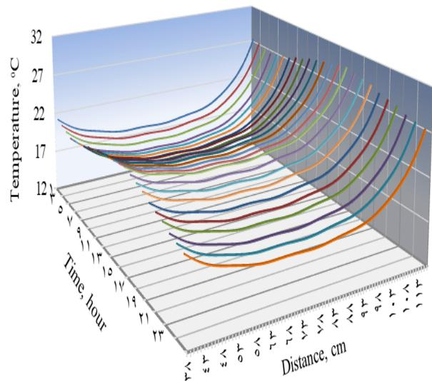
Fig. 7. Variations in temperature within the wall for five pipes at center of the wall during a day
