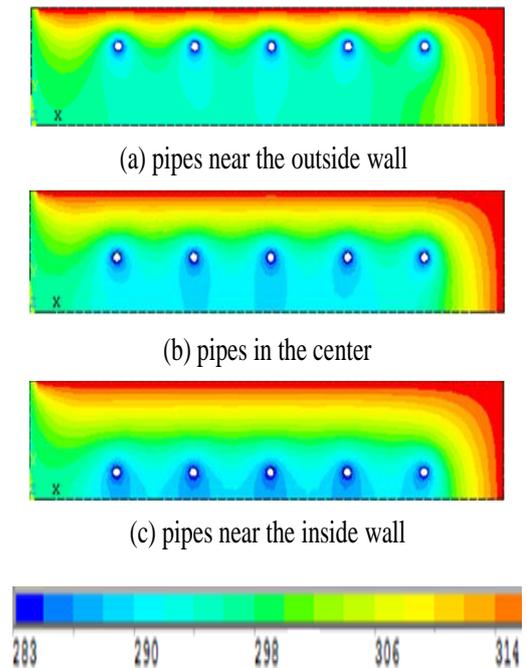
Fig. 10. Temperature distributions within the wall for various pipes locations
