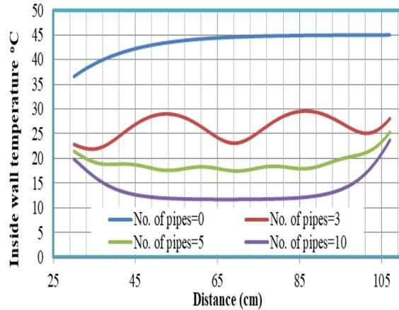
Fig. 9. Variations in temperature inside the wall for all cases regarding the number of pipes
