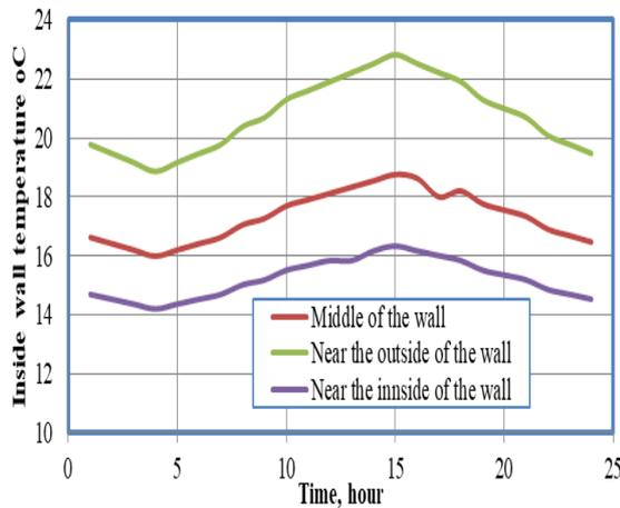
Fig. 12. Variations in the temperature of the wall for various positions of pipes within the wall
