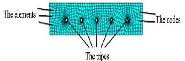
Fig. 3. Meshing of the wall
