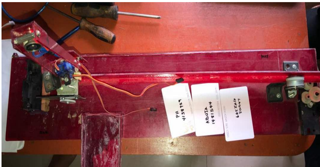
Fig. 13: Hardware Implementation of RFID Airport Luggage Scanning System.
