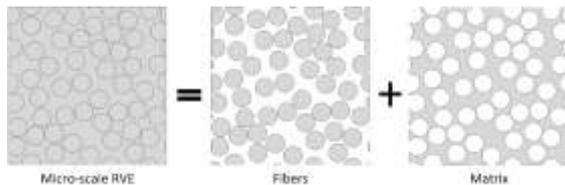
Fig. 1 Geometrical models of composites consisting of randomly distributed fibers and matrix
