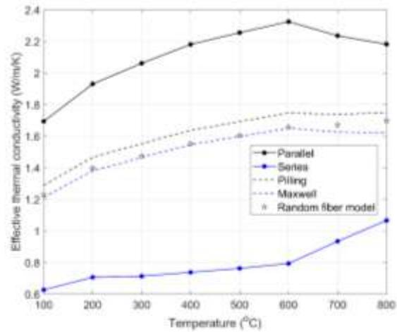
Fig. 5 Comparison of composite thermal conductivity at various temperatures
