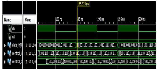
Fig. 13 Simulation result of NoC router for Down port routing operation
