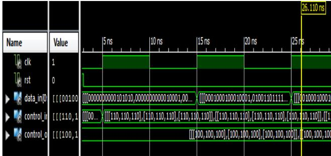
Fig. 10 Simulation result of NoC router for East port routing operation
