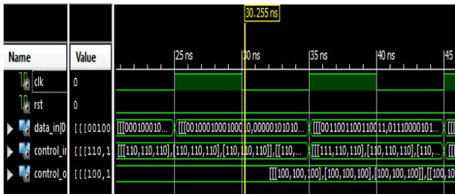
Fig. 11 Simulation result of NoC router for UP port routing operation.
