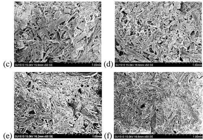
**Fig. 5: Surface morphology (SEM) of oil palm residue handsheet images (50x magnification), (a) OPL untreated, (b) OPL treated, (c) OPT untreated, (d) OPT treated, (e) EFB untreated, and (f) EFB treated.**
