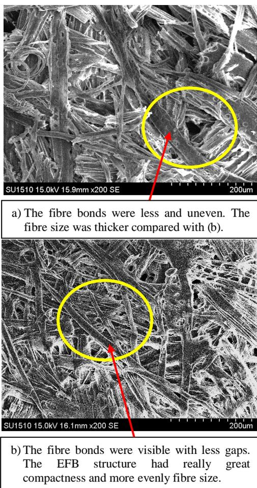
**Fig. 6: Empty fruit bunch (EFB) 200x magnification of scanning electron microscope surface morphology, (a) untreated EFB, and (b) treated EFB.**
