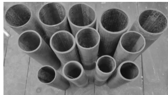
Figure 1. Hollow carbon fiber columns
