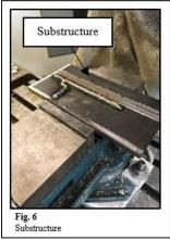
Once the substructure is secure, the CNC (G&M) code to create the part can begin to run which is comprised of the additive and subtractive
