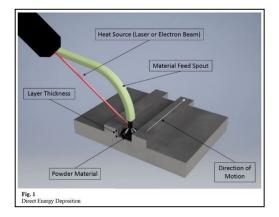
solid layer. This heat source is normally in the form of an electron beam or laser. [5].
