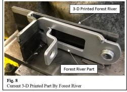
Completion of the part will be when field tests are preformed to ensure proper function at Forest River's manufacturing facility. If the 3-D printed part succeeds, experiments and testing will move forward with future Forest river products along with other companies that want to venture and prototype with this technology.
