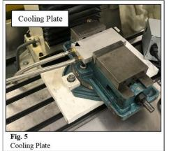
implemented to disperse the heat therefore minimizing the warpage. Without this cooling plate, substructure warpage reaching one quarter of an inch has been observed. In addition to the cooling plate, a measuring device, such as a precise touch probe and a 3-D laser scanner, will be tested to optimize the additive and subtractive manufacturing process.
