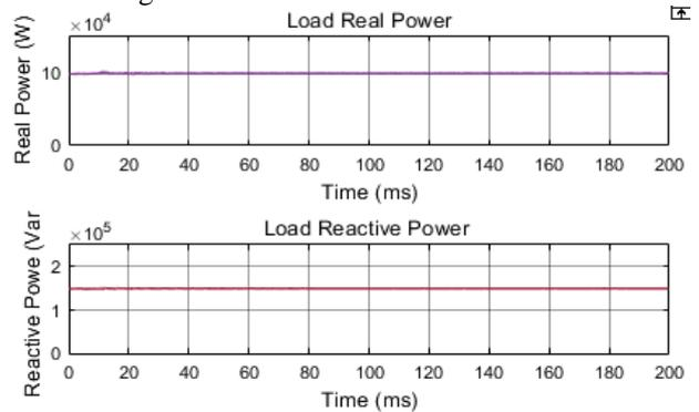
**Fig. 27 Load reactive power and real for case 3.**
