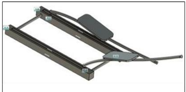
Fig.6 Rail and connecting rod attachment
