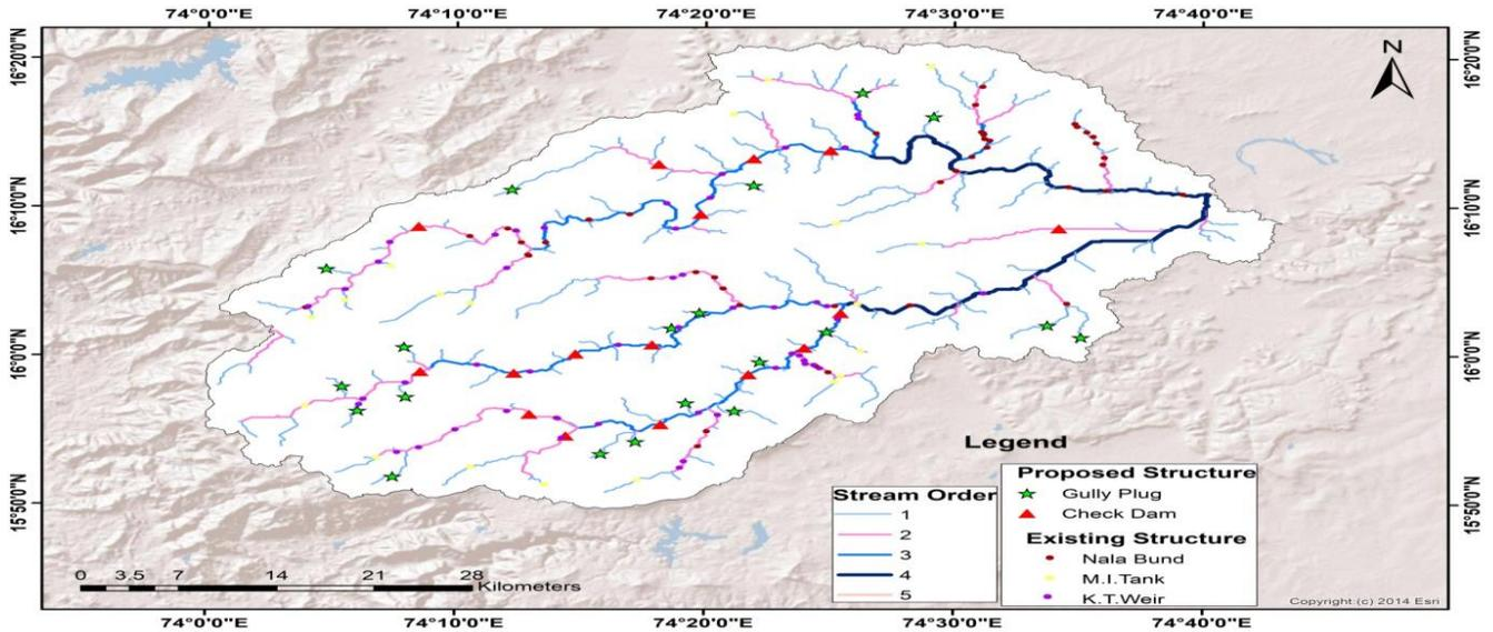
**Fig.18 Existing and proposed soil conservation structure in Ghataprabha Watershed**
